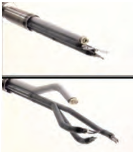
Figure 12-4. The instrumentation articulates at the distal end of the robotic arm, providing complete freedom of motion with scissors, clamps, and cautery. (50)
